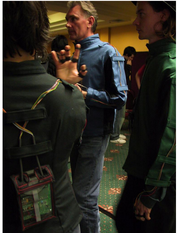
Image 2. Micro-controller location on the back of the jacket
